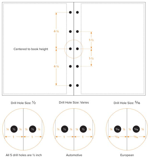
Automotive: First and last drill holes are  $\frac{1}{2}$  inch, other 3 drill holes are  $\frac{3}{8}$  inch.
